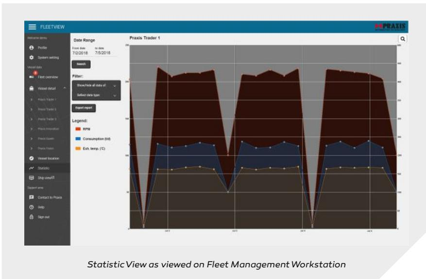
The Statistic View enables the user to print a set of selectable vessel specific parameters over a definable timespan.
